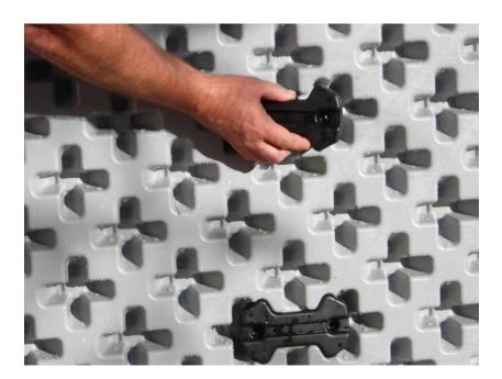
Locate the adjoining pockets on each module and insert connectors into adjoining pockets. Apply downward pressure to lock them in place.
